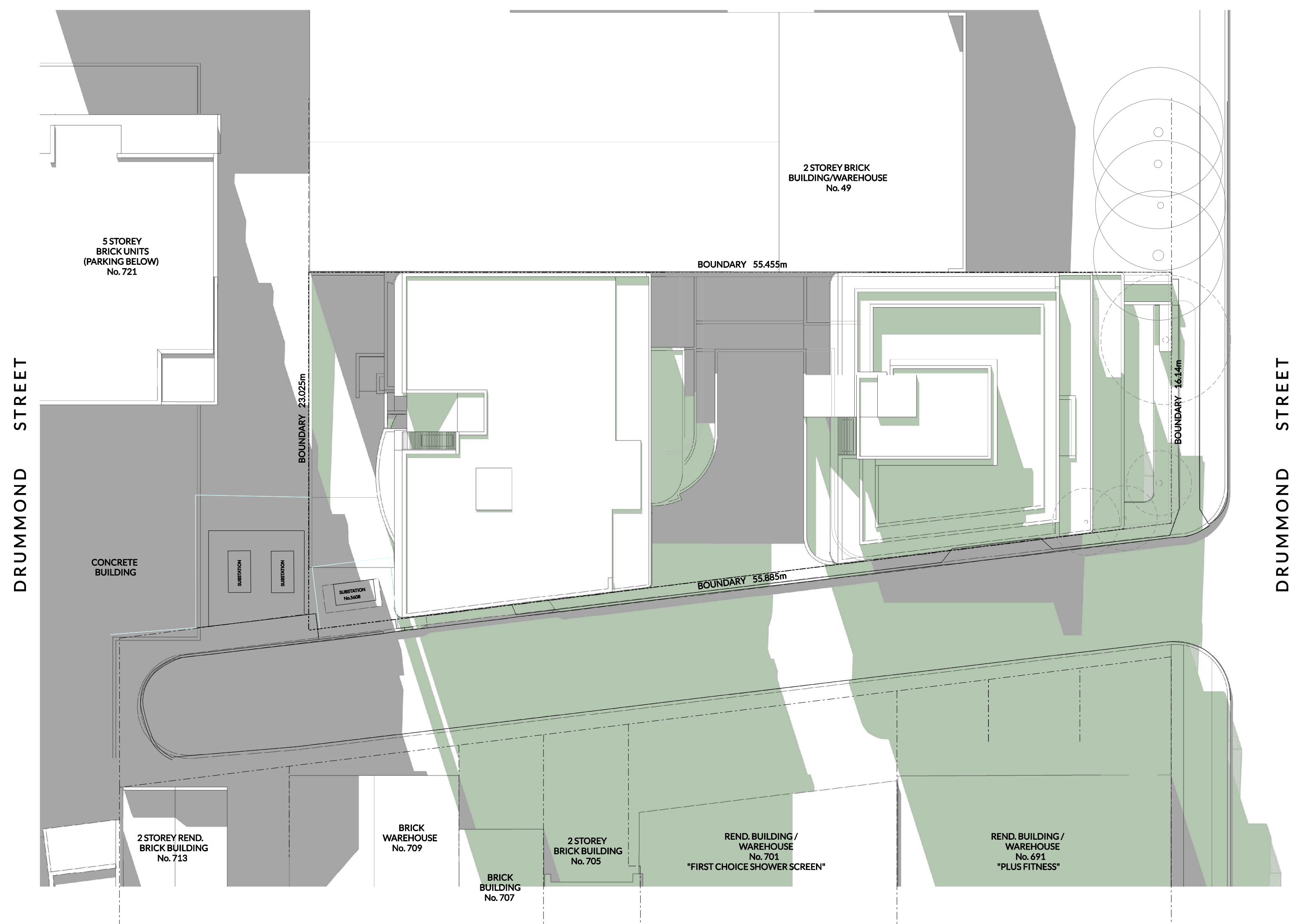
02 SHADOW DIAGRAM - 21 JUNE 3 PM SCALE 1:400 @ A3
